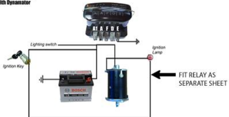
Control Box RB106 With Dynamator
