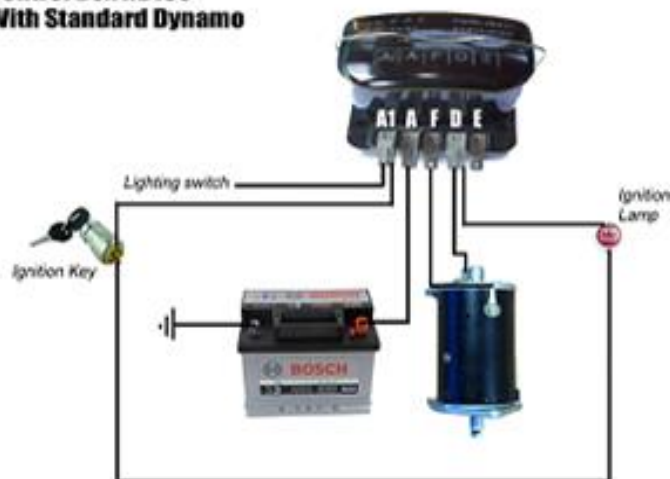
Control Box RB106 With Standard Dynamo
